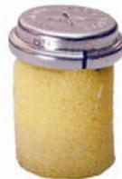
strip that sticks out above the rim with a knife as shown on the right. Before the glue is hardened completely press the strip **firmly** onto the side of the rim with a rod (metal or other material), especially where the diode is soldered onto the metal sticker and the rim.
