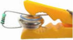
After the cell has been discharged the cell can be emptied. Because of health risks it is advisable to take some precautions. Drilling and removing the insides of the cell is best done in a very well ventilated area or outdoors. Make sure to use household or surgical gloves. Avoid any contact with the insides of the cell with your skin or other body parts. This way health risks are kept to a minimum. These precautions apply until the battery casing has been washed and dried.
