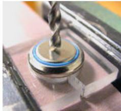
Next, the 3 mm hole must be made larger. Use a 6 or 7 mm drill. After this, you can proceed to the 10 mm drill.
