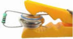
After the cell has been discharged the cell can be emptied. Because of health risks it is advisable to take some precautions. Drilling and removing the insides of the cell is best done in a very well ventilated area or outdoors. Make sure to use household or surgical gloves. Avoid any contact with the insides of the cell with your skin or other body parts. This way health risks are kept to a minimum.
