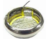
Loosen the "flap" of the conductive foil from the rim of the battery casing. Solder the wire from the anode of the Schottky diode onto the loosened "flap" of the conductive foil at the spot where the "flap" falls in the rim of the battery casing, as shown on the left. Try to do this in less than 0.5 seconds so the wire won't come off the Schottky diode while soldering. (see: **TIP Utility knife** on page 6).
